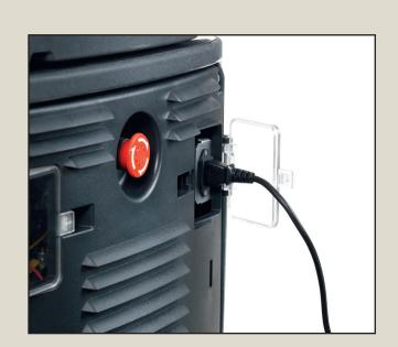
Disconnect battery charger and store the cable in the storage compartment located under the seat.
