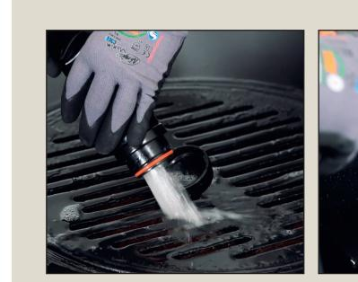
Empty and clean the recovery tank and float system.
