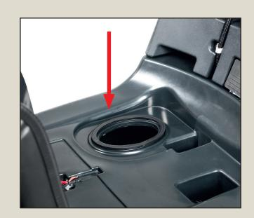
Fill the solution tank with fresh water and add low foam detergent according to needs.
