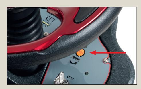
Switch brush motor button on.
