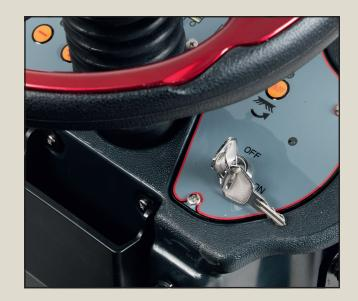
Turn OFF the machine using the key.
