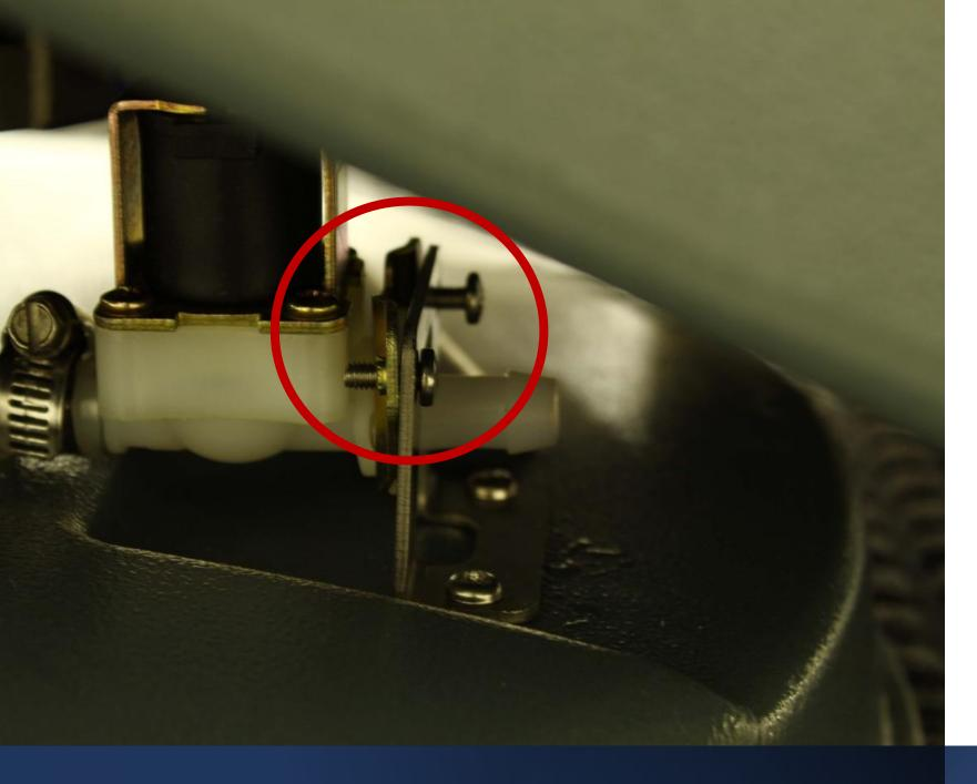
1. Remove the 2 Philips head screws holding the solenoid to the solenoid bracket
