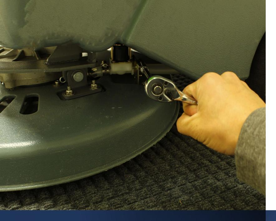
Remove the hose clamps by turning counter-clockwise using a 7mm socket or flathead screwdriver
