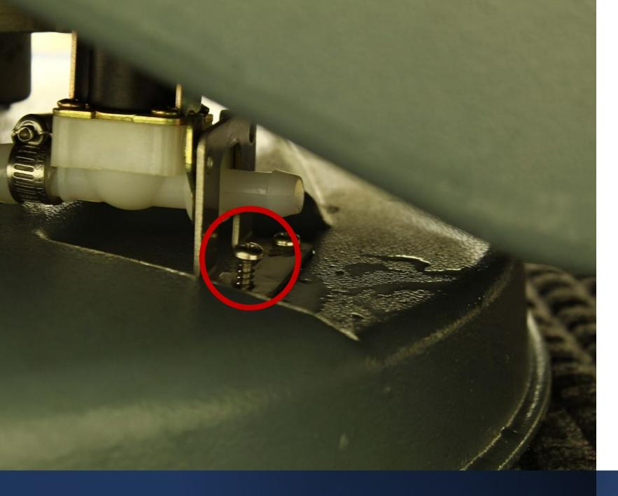
1. Screw in the Philips head screw back into the scrub deck
