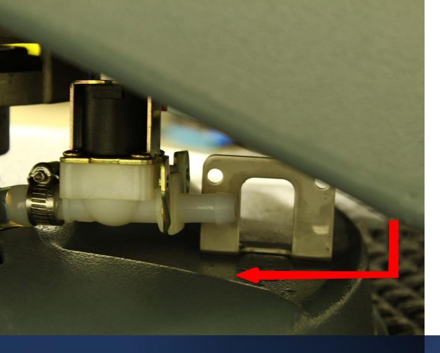
1. Rotate the solenoid backet back to the original position
