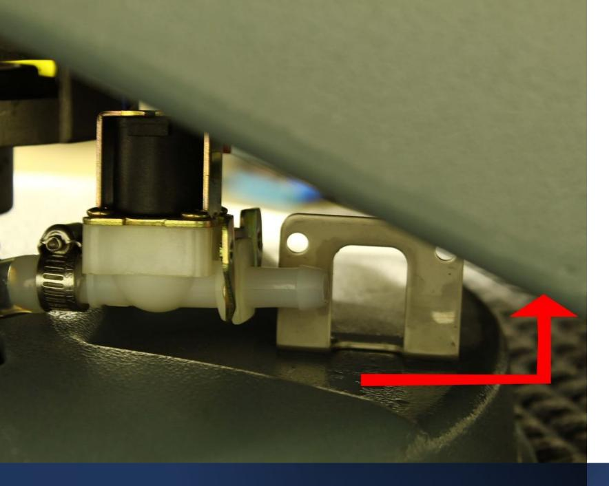
1. Rotate the solenoid bracket out of the way
