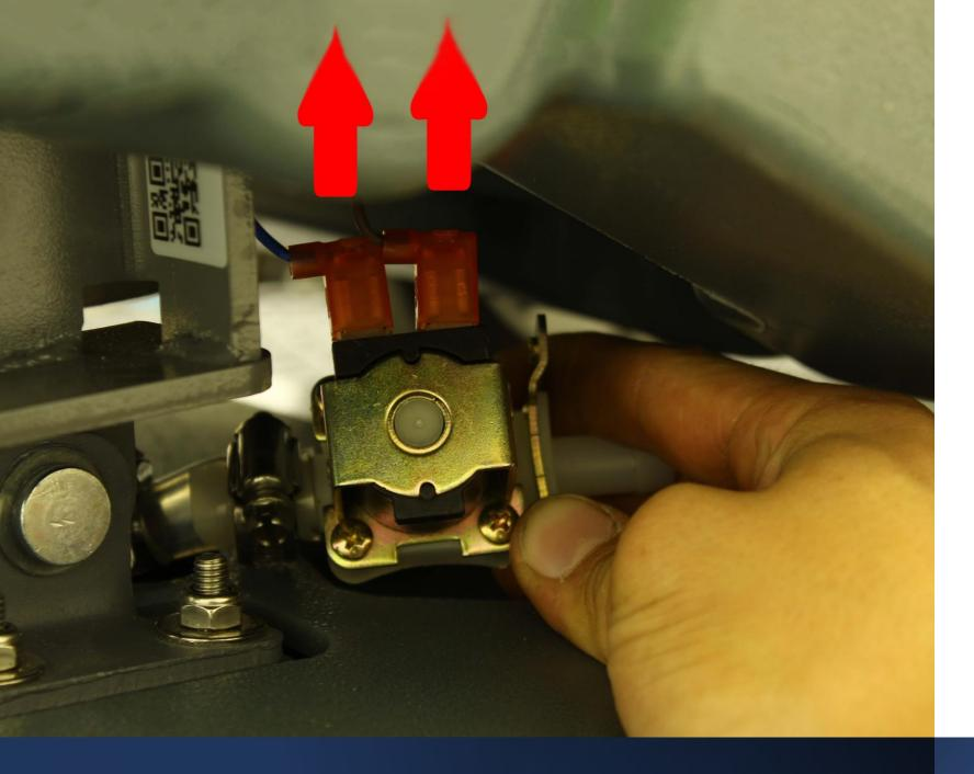
• Remove the 2 Wire connections from the solenoid
