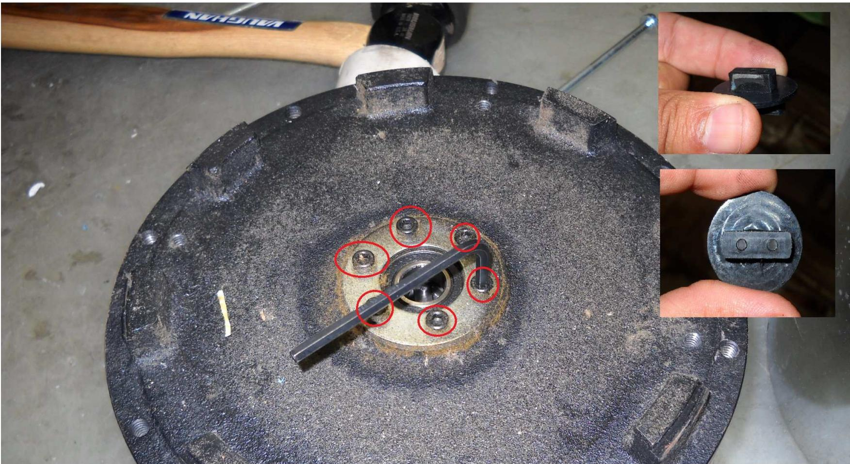
**Step 4. Remove the allen head bolts that are holding the coupler housing plate in place. Remove the plate and the broken coupler and any debris and replace with new coupler. Put the plate back on and tighten the bolts.**
