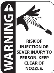
**WARNING:** The high pressure developed by this pressure washer can cause personal injury or equipment damage. Keep clear of the nozzle. Use caution when operating. Do not direct the discharge stream at people, or severe injury or death could result.
