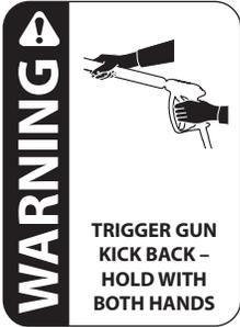
**WARNING:** Grip the cleaning wand securely with both hands before starting. Failure to do this could result in injury from a whipping wand.
