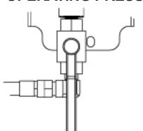
VALVE OPEN: WATER SUPPLIED TO HOSE REEL FOR OPERATION OF PRESSURE WASHER.
