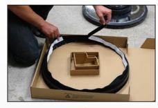
2. Remove VELCRO® with white adhesive backing from the inside of the dust skirt. Then remove the backing from the VELCRO® exposing the adhesive for attaching to the housing of floor machine.
