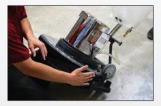
4. Apply the Malish Dust Skirt with vacuum port positioned at the bottom left of the floor machine housing when you are standing in the operator position. This will allow for maximum dust control.
