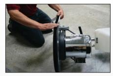
3. Apply VELCRO® strip to the middle/ upper half of the outside diameter of the floor machine housing (bumper).
