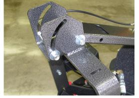
7. Rotate handle to the user position. Then insert the bolt through the handle bracket and handle top.
