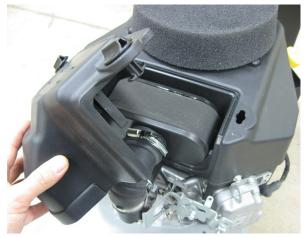
4. Loosen clamp that retains filter and remove the air filter.
