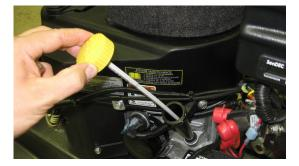
If necessary, place a block under the back of the machine or apply weight to the front of the deck to maintain an upright, level position.
