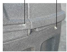
right and left housing latching bolts for open housing section
