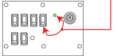
"Circuit test" switch next to the green light, push that switch and the green light should glow. If not it is not on two separate circuits.
