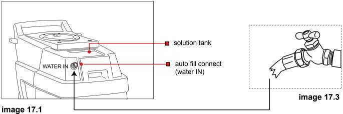
Connect the end with a female Q.C. to the water in (Auto Fill System) on the extractor
