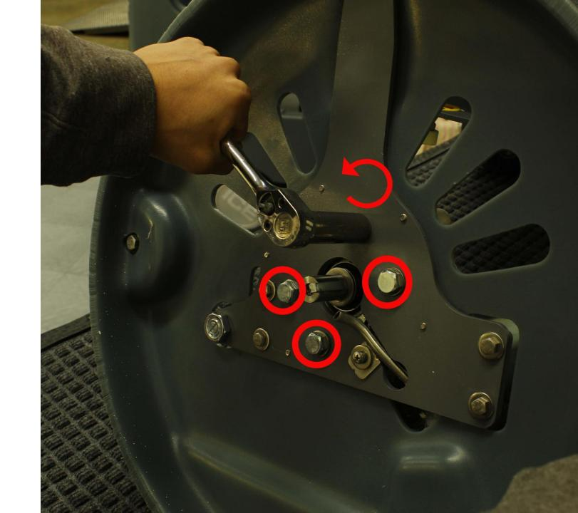
Pull the motor off the scrub deck housing
