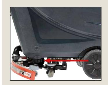
Daily: Empty the clean water tank using the solution tank drain knob under the machine.
