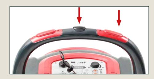
For wheel traction version: pressing either of the red safety switches and the black reverse button together will put the machine into reverse.
