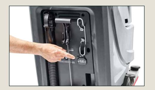
Daily: to charge the battery, use the supplied AC cord to the on board charger and connect it to the machine and wall socket.
