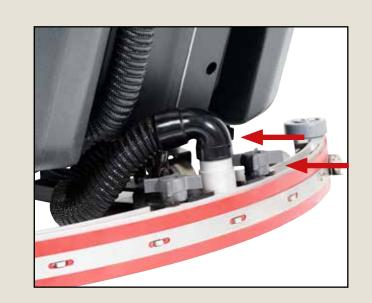
Install the squeegee using the thumb nuts. Attach squeegee hose.
