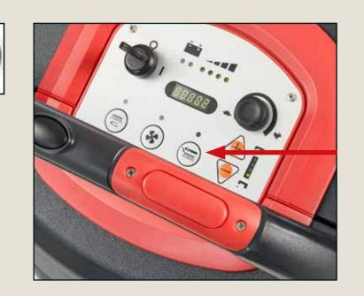
On disc version, the brush/pad holder can be removed automatically by raising the deck with the pedal and then press the click off button.
