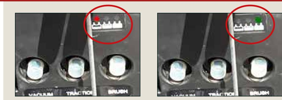
Daily: if the battery indicator shows red, put the machine on charge. Battery should be on charge if empty, not in use or if not being used for coming 8-10 hours.
