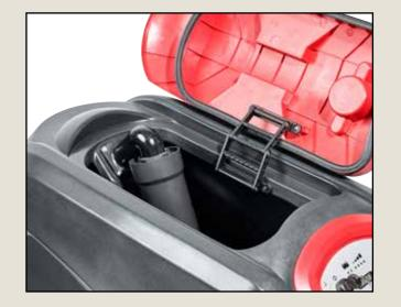
Daily: Inspect and rinse the float ball cage and inspect and clean the lid gasket if required.
