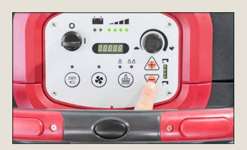
Press the + or – solution buttons to increase / decrease the water flow rate or to turn solution off.
