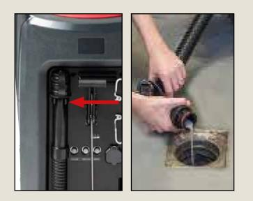
Daily: Empty the recovery tank using the recovery empty hose. Bend the soft part before removing the cap to control the flow.
