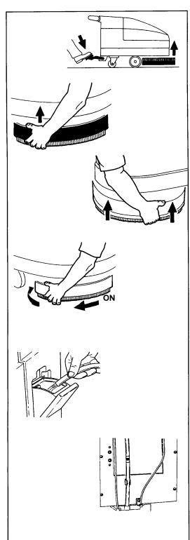
Center the pad brush on top of the holder and replace the locking device. The locking device should be tight.
