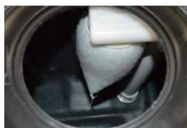
vacuum filter and ball float cage in recovery tank
